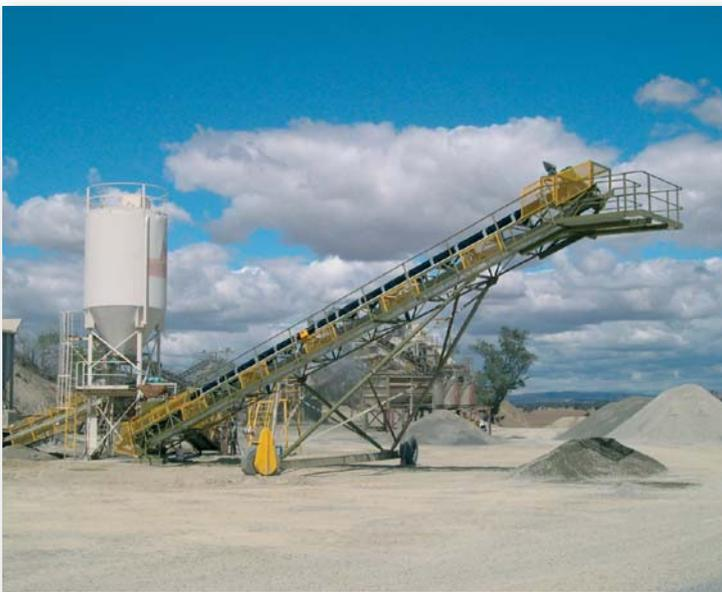
In an effort to improve production and sales efficiencies with its wet mix products, Yabba Quarries put forward a proposal for a radial stacker to reduce double handling of products and the need for long hours to prepare for up to 5 different wetmix products, to be made and loaded in the one day.
