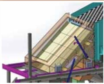
3D model of roll out chute showing flop gates and modular wear panels.
